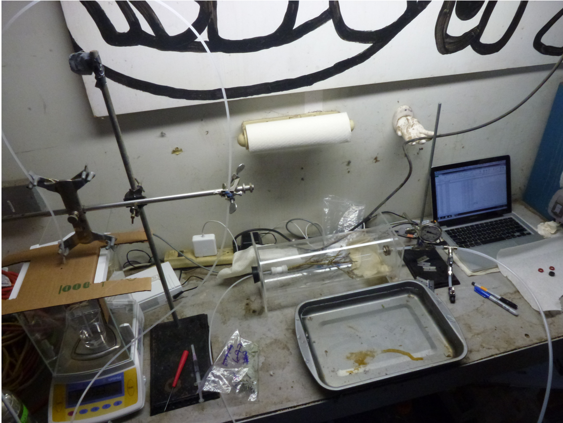
Figure 6: Apparatus for measuring stem hydraulic conductance.
