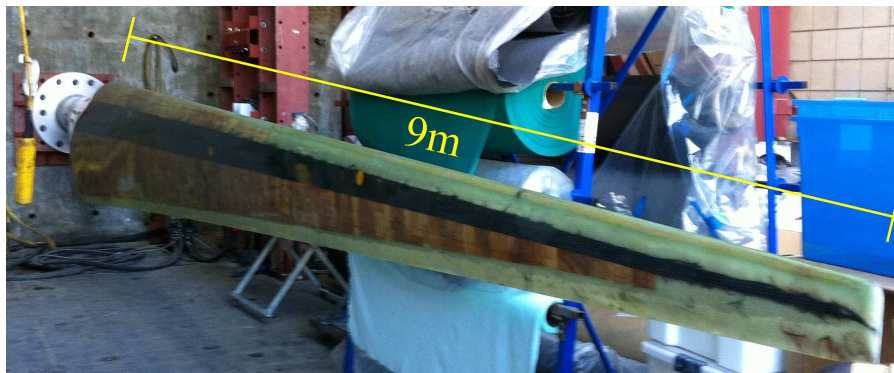
Figure 3.1: The CX-100 blade cantilevered at the UCSD Powell Labs
