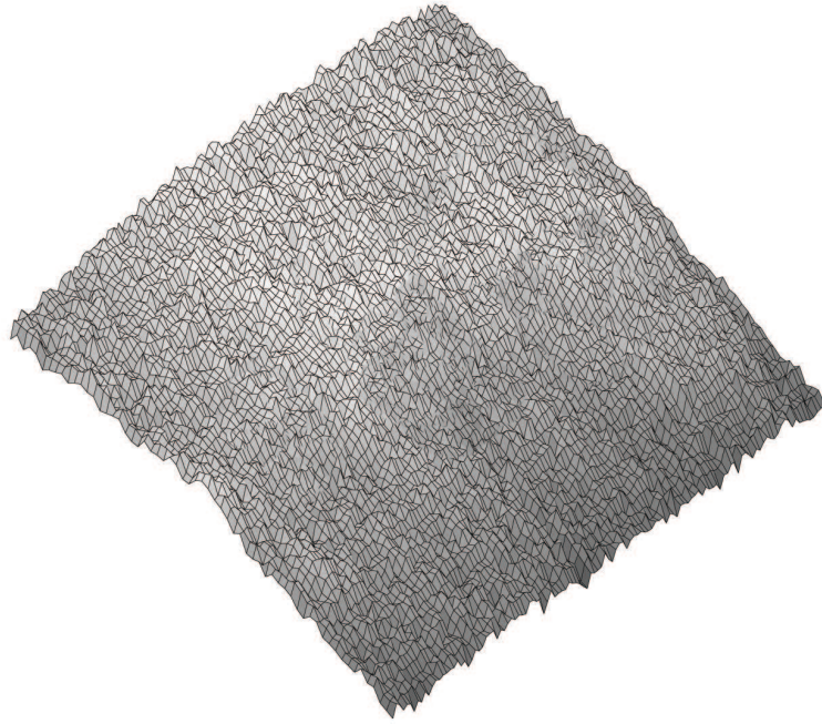
Figure 2.14: 3D surface view of the wavelet filtered data obtained on sandwich plate with disbonds, 0.5s after flash input
