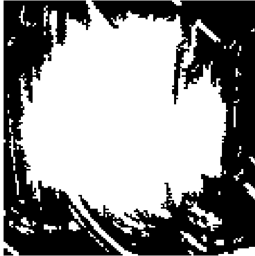
Figure 3.9: Sequence of image processing steps performed on a phase image obtained over an area containing a 50.8mm diameter skin-skin delamination at a depth of 1.3mm from the blade surface. Binary image that is obtained by thresholding the scaled intensity value at 0.7, followed by application of morphological operations
