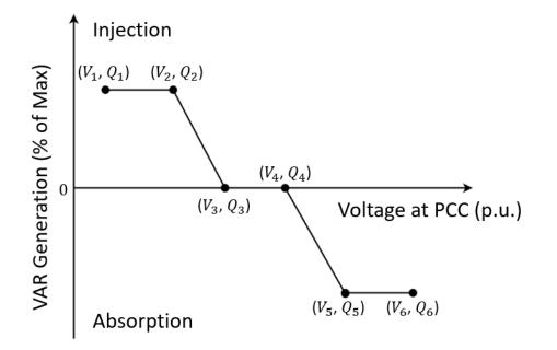
Figure 4.1: A typical Volt-Var droop curve of a smart inverter.
