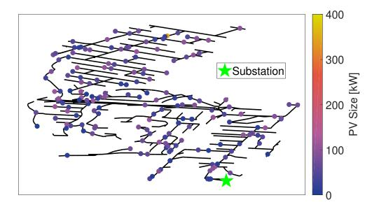
**Figure 3.3**: Feeder topologies of the California utility feeder. Black lines represent feeder lines. Each dot is a PV system and its color indicates its AC power rating. The OLTC is located at the substation (green star).
