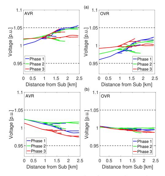
**Figure 3.6**: Feeder voltage profile at 11:32 (top, a) and 21:00 (bottom, b) for the AVR (left) and OVR (right) voltage regulation methods.
