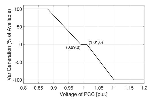
**Figure 3.4**: Volt-Var curve of SI adapted from [5]. The SI injects/absorbs the corresponding percentage of available vars based on the voltage at the point of common coupling (PCC). The available vars  $(Q_{max})$  are limited by PV real power generation and SI rating as shown in Fig. 4.2.
