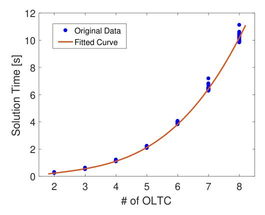
**Figure 2.8**: Computation time for the optimization (excluding power flow) for one time step as a function of total number of OLTCs.
