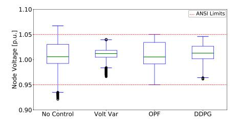
Figure 4.9: Boxplot of node voltages of the 1 year test with 8760 scenarios on the IEEE 37 bus test feeder. For each case, the boxplot contains voltages of all nodes of all 8760 test scenarios (324,120 data points). Red dashed lines represent the [0.95,1.05] p.u. ANSI limits [7].
