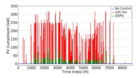
Figure 4.12: Total PV generation curtailment of each scenario/step of three different cases for the IEEE 123 bus feeder.
