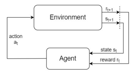
Figure 4.3: Schematic over-view of reinforcement learning.
