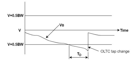
Figure 1.2: Illustration of autonomous operation of OLTCs. The OLTC monitors its local bus voltage  $V_B$ . If the local bus voltage deviates from the preset reference voltage V outside of the allowable range (0.5BW, half of dead band) for a duration longer than the time delay  $(T_D)$ , the OLTC will adjust its tap position to bring the local voltage back within  $V \pm 0.5BW$ .
