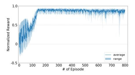
**Figure 4.7**: Reward during training process for the IEEE 123 bus feeder. The dark blue line represents the average reward of 5 experiments with different random seeds, and the shaded light blue area display the range of episode average reward (average of rewards of all iterations in the episode) of those 5 experiments.
