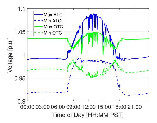
Figure 2.5: Time series of maximum and minimum voltage of feeder B with 150% PV penetration on March 14, 2015.
