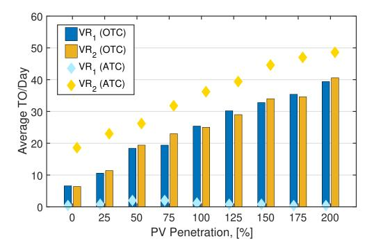
Figure 2.7: Average TO/day of each OLTC on feeder B over the 28 day simulation period as a function of PV penetration.
