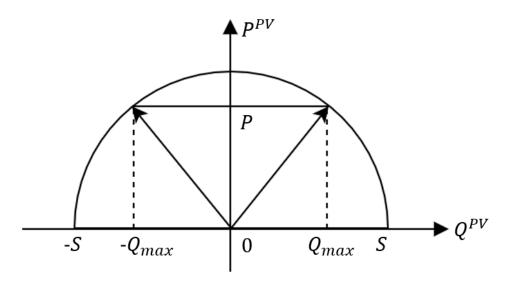
Figure 3.1: PV smart inverter output curve. P is the PV real power production, which is determined by the solar irradiance at each time step. Assuming no curtailment, given the SI rating S, the reactive power output can then vary between  $-Q_{\text{max}}$  and  $Q_{\text{max}}$ .
