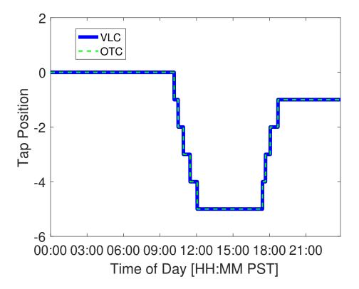
Figure 2.4: Time series of the tap position on feeder A with 200% PV penetration on March 14, 2015.
