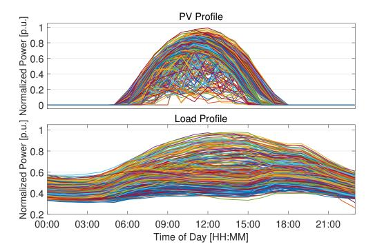
**Figure 4.8**: Normalized PV (top) and load (bottom) profiles used for tests. The PV generation profile is from public solar power datesets maintained by NREL [6]. The load profile is from the OpenDSS installation directory [2]. Single profile is used for all PVs and loads. 1 year (365 days) profiles are plotted here.
