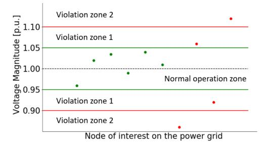
**Figure 4.5**: Definition of voltage profile zones. Each dot represents voltage of one node. The corresponding total voltage reward for this example is  $2 \times Penalty_1 + 2 \times Penalty_2$ .
