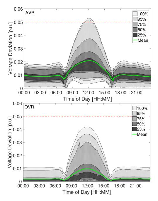
**Figure 3.9**: Distribution of absolute values of feeder nodal voltage deviation from 1 p.u. for AVR (top) and OVR (bottom) cases.
