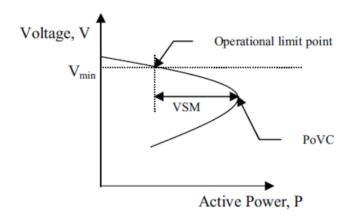
Figure 5.1: P-V nose curve.
