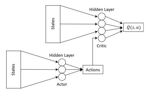
**Figure 4.4**: Deep deterministic policy gradient network. The actor suggest actions based on received states. The critic evaluates the actions provided the current states.
