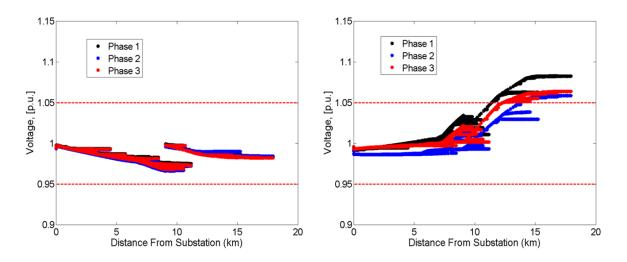
Figure 1.4: Voltage profile of the distribution feeder in the middle day with 0% (left) and 150% (right) PV penetration using autonomous voltage regulation. The red dash lines indicate the [0.95, 1.05] p.u. ANSI limits. The substation is at the feeder head and PVs are located downstream on the feeder. PV penetration is defined as the ratio of total PV installation capacity and peak demand on the distribution feeder.
