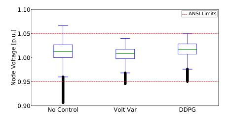
**Figure 4.11**: Boxplot of node voltages of 1 year test with 8760 scenarios on the IEEE 123 bus feeder. For each case, the boxplot consists of voltages of all nodes of all 8760 test scenarios (1,121,280 data points). Red dashed lines represent the [0.95,1.05] p.u. ANSI limits [7].
