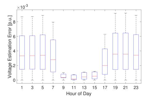
Figure 3.5: Box plot of voltage estimation errors for the IEEE 37 bus test feeder. For readability, the results are aggregated over two hours into 12 groups.
