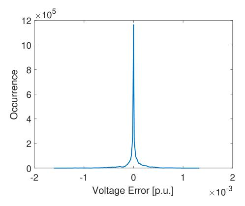
**Figure 2.3**: Distribution of voltage errors from the fixed current injection assumption, linearization of admittance matrix, node voltages. The distribution is created from simulations for feeder B with 150% PV penetration.
