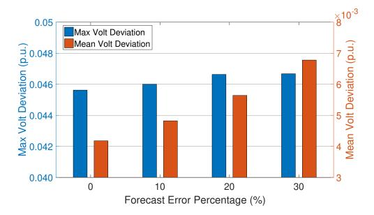
**Figure 3.10**: Maximum and average voltage deviation of the IEEE 37 bus feeder under different levels of forecast errors with OVR. Both quantities are calculated based on all nodal voltages for simulations of the same cloudy day as Section 3.5.2
