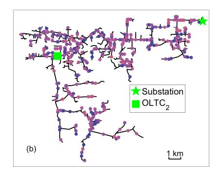
**Figure 2.2**: Feeder topologies of feeder (a) A and (b) B. Black lines represent feeder lines. Each dot is a PV system and its color indicates its AC power rating. The substation is marked with a green star and the green square marks the additional OLTC of feeder B.
