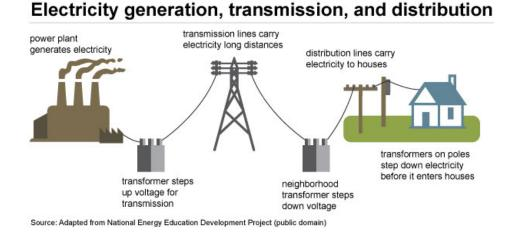
Figure 1.1: Electricity generation, transmission, and distribution.
