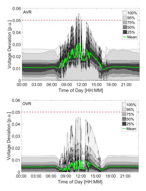
Figure 3.7: Distribution of the absolute values of feeder nodal voltage deviations from 1 p.u. for all nodes on the IEEE 37 bus feeder. top: AVR; bottom: OVR. The absolute values are plotted for consistency with  $J_1(3.21)$ . The red dashed line represents the [0.95 1.05] p.u. ANSI voltage limits. For the IEEE 37 bus feeder, all voltage deviations greater than 0.05 are over-voltages.
