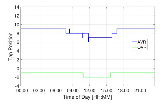
Figure 3.8: Time series of OLTC tap positions  $\tau$  for the IEEE 37 bus feeder.
