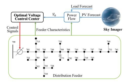
Figure 2.1: Structure for proposed optimal voltage control.
