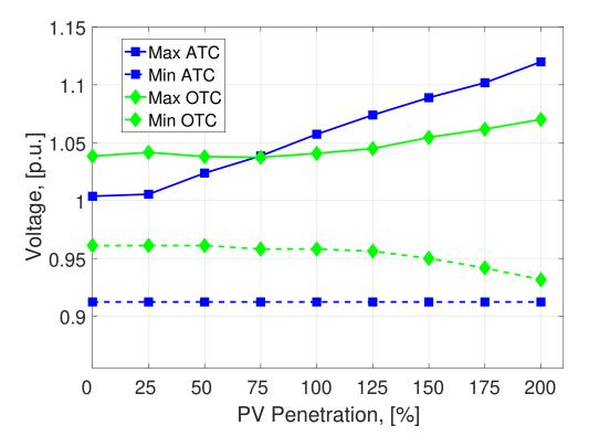
**Figure 2.6**: Maximum and minimum voltage as a function of PV penetration level on March 14 2015 for feeder B.
