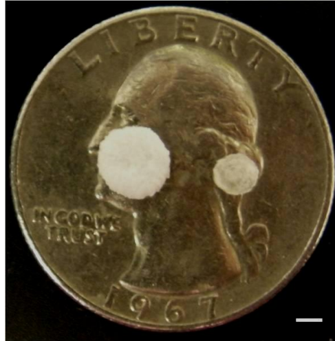
Figure 9. A feasibility study to show the use of natural polymers for shrinking is shown with an ethylcellulose net-shape scaffold (left) and shrunken fibrin scaffold (right). The ethylcellulose was used as a sacrificial material for the final fibrin scaffold. The dried fibrin scaffold has not been processed with a secondary treatment to retain shrinking. Scale bar is 2 mm.
