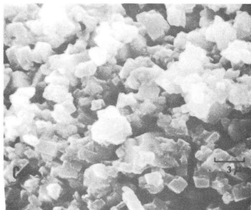
Fig. 27. Scanning electron micrograph showing decrease of grain size due to an increasing amount of barium doped into material prepared with nitrates.
