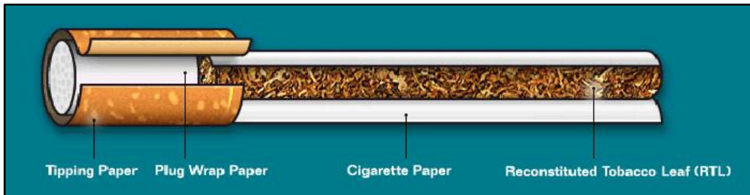
Fig 1.1. Schematic diagram depicting the parts of a tobacco cigarette. (From Smoker News World)
