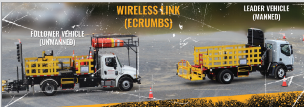
FIGURE 5. ATMA in Operation (source: AHMCT)
