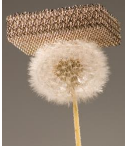
Figure 3: Nickel microlattice, example of architected material [22].
