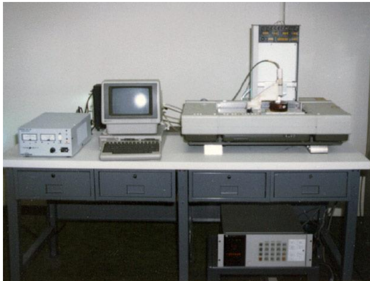
Figure 5: One of the first stereolithography machines ever made [30].
