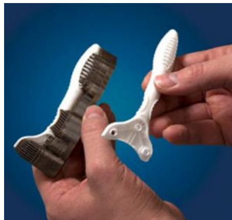
Figure 6: Example of part printed with a different support material [35].
