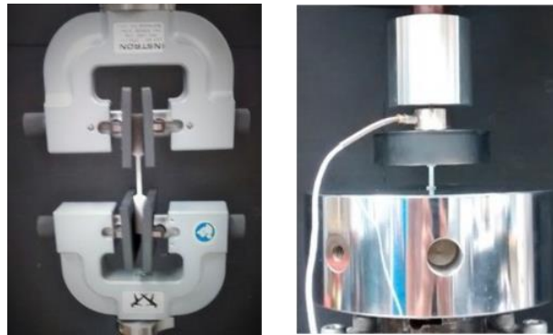
Figure 10: Tensile (left) and compressive (right) tests of a bar.
