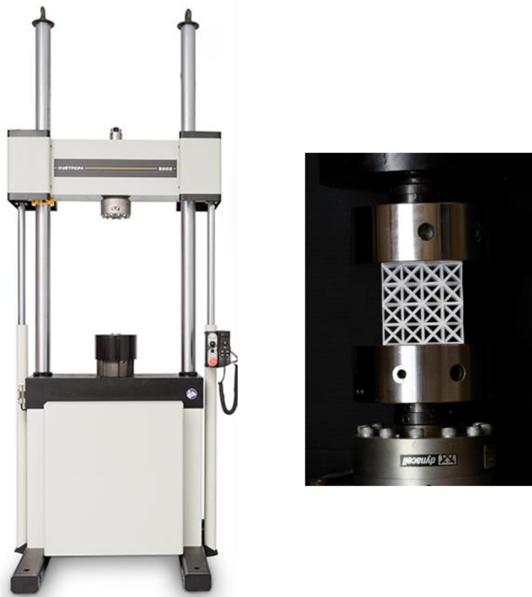
Figure 15: INSTRON 8862 used to perform the tests (left) [53] and sample being tested (right).
