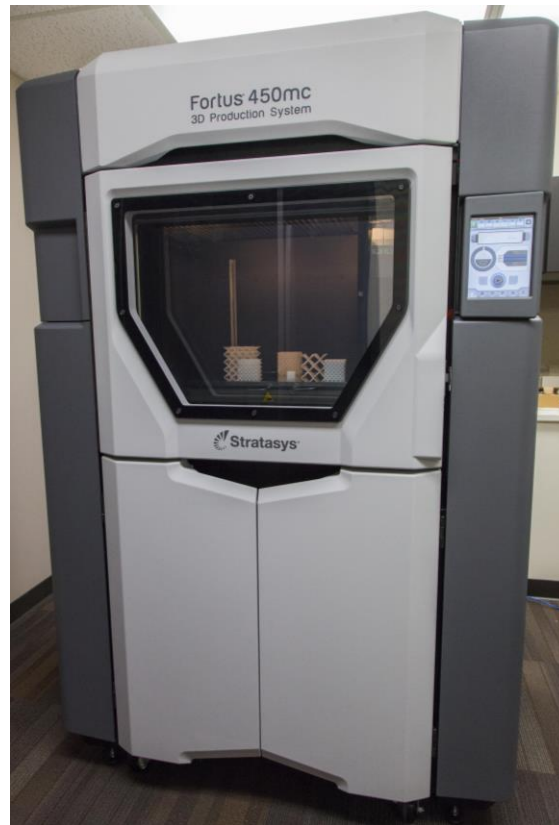
Figure 8: Stratasys Fortus 450mc fused deposition modeling 3D printer.
