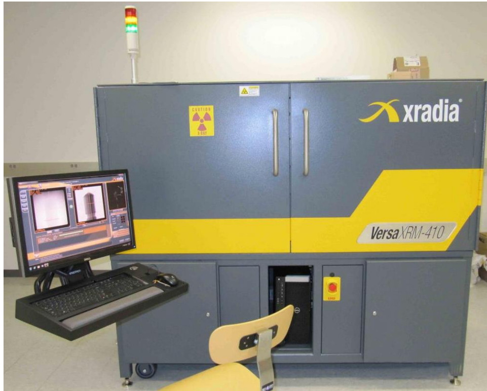
Figure 11: X-ray CT scanner Xradia VersaXRM™ 410.
