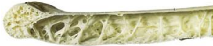
Figure 1: Cellular material in the core of a bird bone [2].
