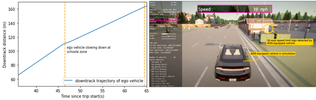
Figure 5.6: Trajectory plot and the simulation screenshot when ego ADS vehicle adjusting speed for areas with different speed limit regulations.
