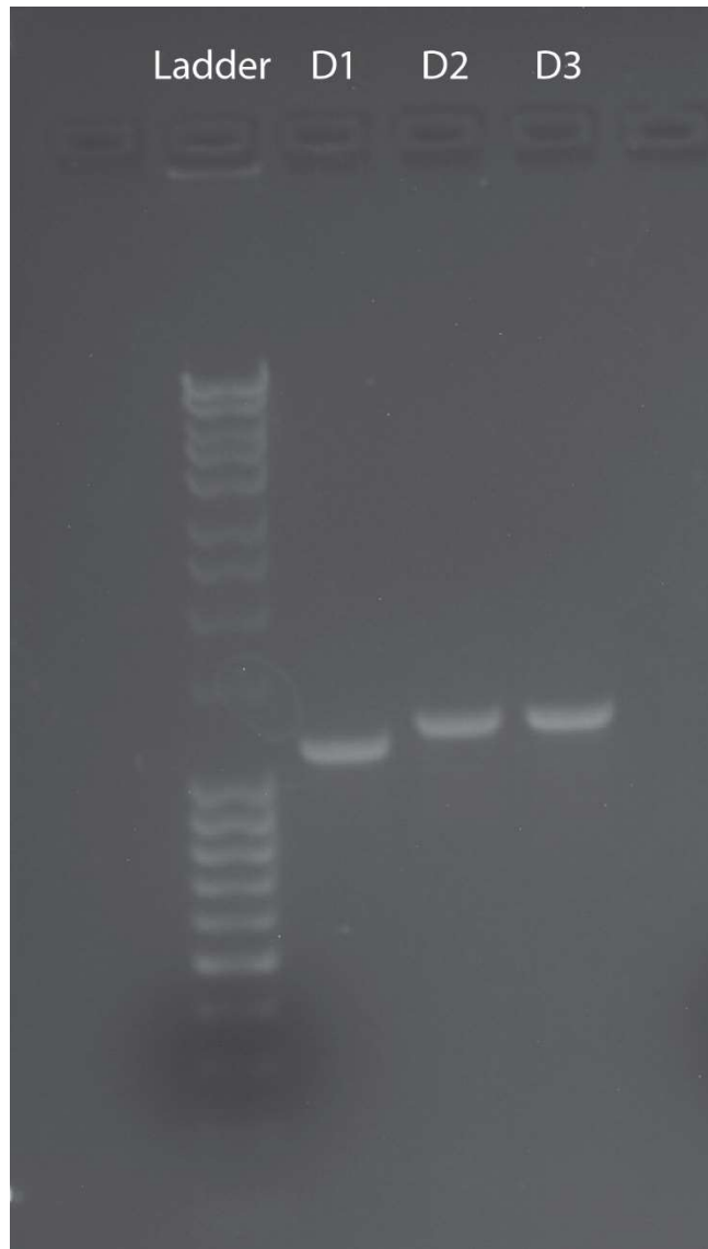
Figure 5.2. Validation of isolated decorin cDNA genomic size before gene sequencing. Three different primers designs were utilized for decorin cDNA isolation based on the available sequence in EquCab3.0. The gel confirmed cDNA isolation of decorin in the expected range.
