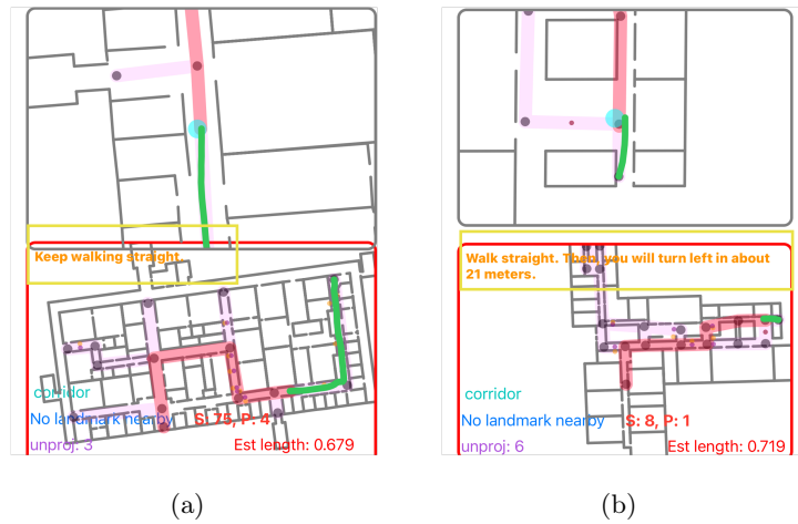
Figure 5.15: Notifications for passing through Non-Turning Junctions (NTJs), highlighted within the yellow box for S2. (a) Activation of the S2 state, and (b) Activation of both the S1 and S2 states. The pink lines indicate the optimal route, while the green lines track the user's actual path. The cyan dot represents the user's projected location on the associated segment.
