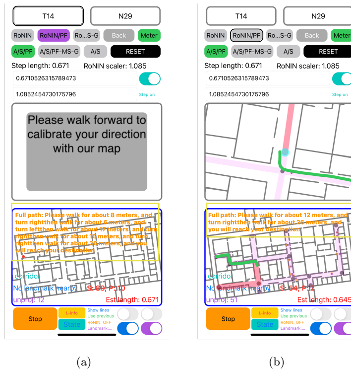
Figure 5.21: Notifications for the "swipe left" gesture on the watch during navigation. (a) The complete path is generated based on the optimal route from the starting point to the destination, marked by a highlighted yellow box. (b) When on the route, performing a "swipe left" gesture generates navigation instructions for the full path from the current position to the destination point, also marked with a highlighted yellow box.
