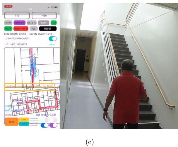
Figure 5.24: (a)–(b) Recorded route R1W using A/S (blue line) and RoNIN (red line) for (a): P1. (b): P2. (c) Synchronized screenshot of the app and P4’s perspective, as he notices the staircases on his right side. The notification generated by the app is highlighted within an orange box. Experimenters reminded him to avoid ascending the stairs.
