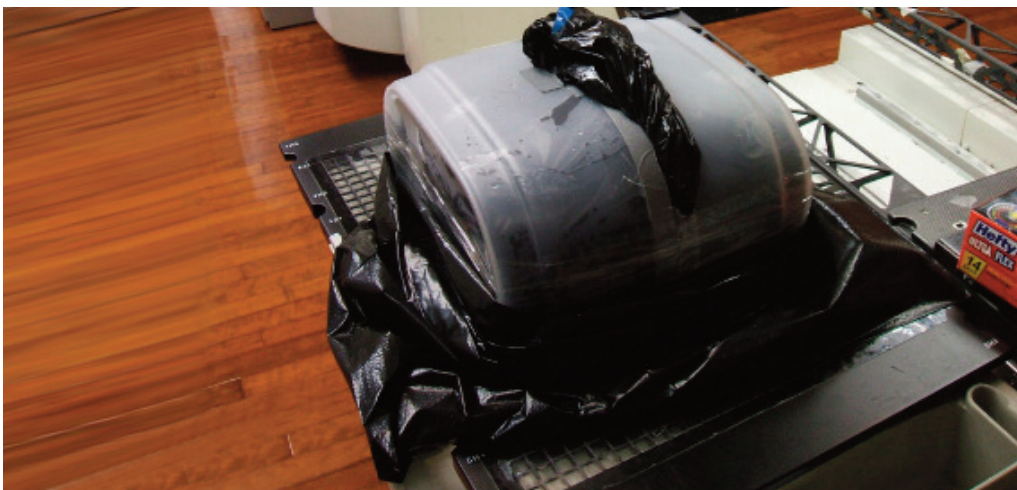
FIG. 2. Example of a custom-made pelvic water phantom. This picture shows phantom B.
