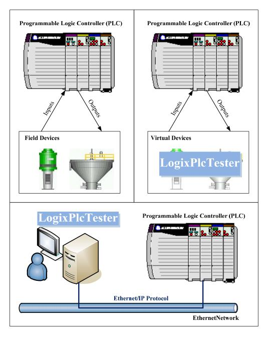
Figure 4.1: LogixPlcTester design concept diagram.
