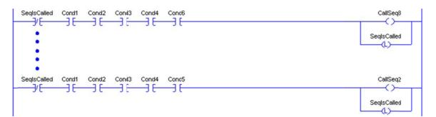
The bug in the above ladder code is introduced by a weak trigger condition for a sequence. A possible solution is to tighten the trigger condition for Sequence 8 as follows:
