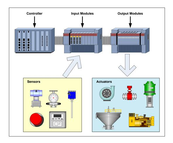
Figure 1.1: Typical PLC configuration.
