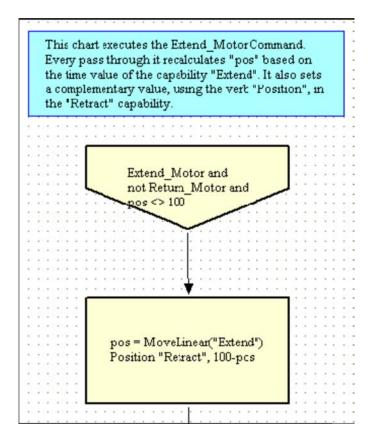
Figure 6.2: RSTestStand flowchart.
