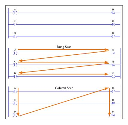
Figure 5.8: A code example for demonstrating scan methods.
