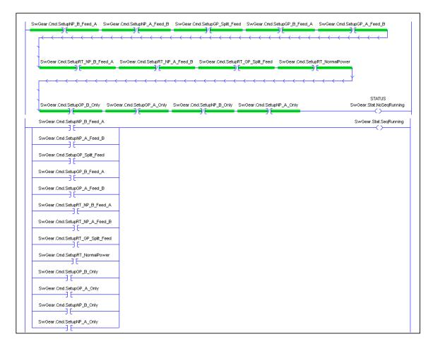
Figure 5.13: Fixes for the ladder code in Figure 5.12.
