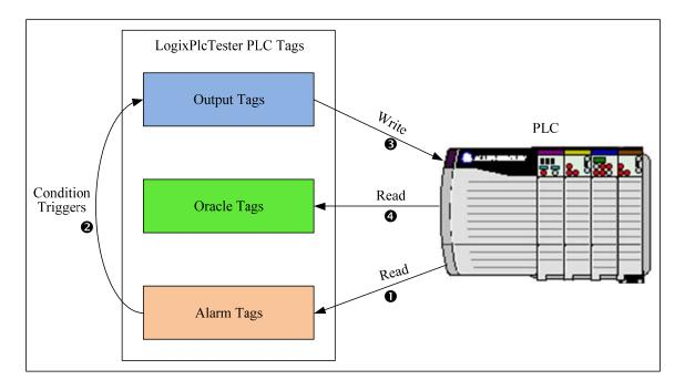
Figure 4.17: LogixPlcTester data flow path.
