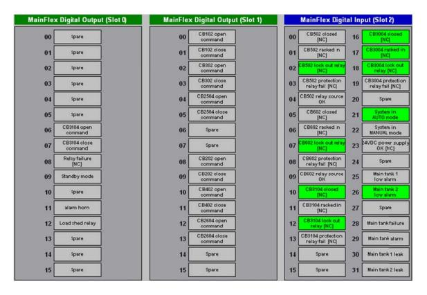
Figure 3.2: Allen Bradley PanelView I/O simulation screen.
