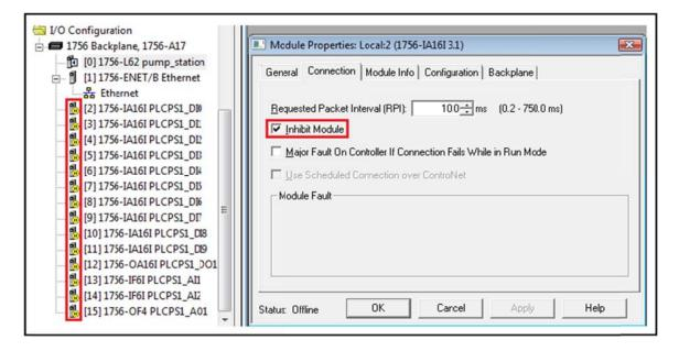
Figure 4.2: Inhibit PLC I/O modules.
