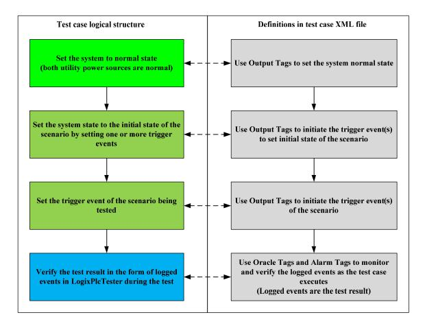
Figure 5.3: Logical structure of a LogixPlcTester test case.
