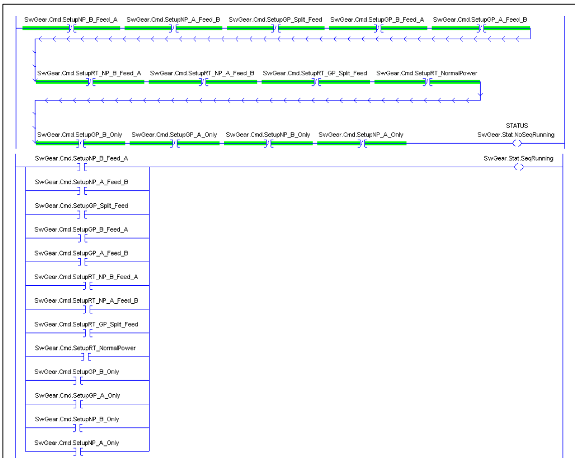
Figure 5.13: Fixes for the ladder code in Figure 5.12.
