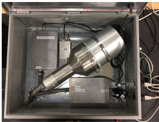
Figure 4.3: A single 5"×5" plastic scintillator mounted to a photo multiplier with accompanying high voltage and signal processing electronics. This instrument was first deployed at the Säntis Tower in Switzerland during 2020 and 2021. It is currently deployed on the Dalmatian coast in Split, Croatia.
