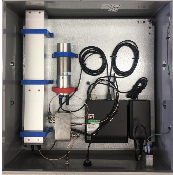
Figure 4.5: The Airborne Detection Of Thunderstorm Radiation (ADOTR) instruments consist of a two detector array. The array consist of one plastic scintillator and one sodium iodide scintillator each mounted to a photo-multiplier tube (PMT). The analog shaping and digitizing electronics are incorporated into the high voltage base of the PMTs. The shaped waveform is sampled by a 40 MHz ADC with an FPGA acquiring and managing the data, while an ARM processor controls the PMT and executes gain and performance stabilization. The detector electronics interface with the instrument computer via USB 1.2, and the 5V USB hub power is used by the detector base to supply the necessary high voltage to the PMTs. A total of 10 instruments are being deployed on separate C-130 USAF Hurricane Hunter Aircraft.
