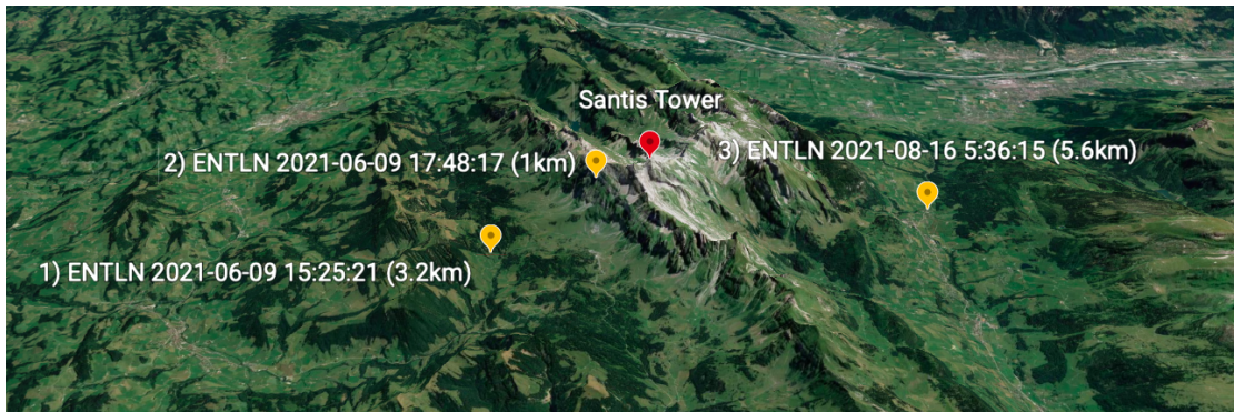
Figure 3.1: Earth Networks Total Lightning Network (ENTLN) geo-locations (yellow markers) for each event and distance from the Säntis Tower (red marker)
