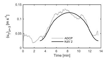
Figure 2.8: Total cross-shore velocity  $[m s^{-1}]$  at 3-m depth. The grey line shows 30-s smoothed ADCP measurements, while the black line shows the scaled KdV 2 velocities (Fig. 2.7).
