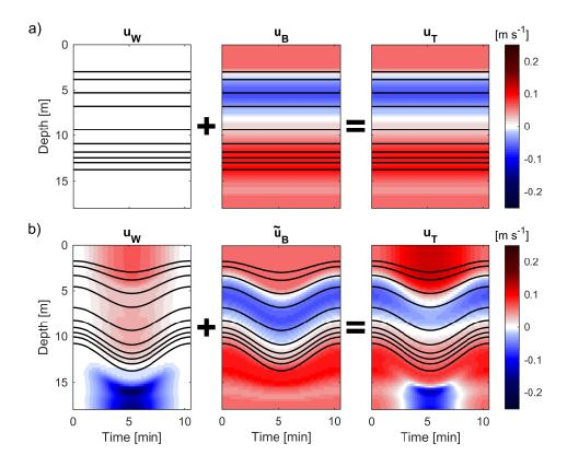
**Figure 2.3**: Wave and background contributions to total cross-shore velocities,  $u_T$  [m s<sup>-1</sup>]. a) Unperturbed background,  $u_B$ . b) Wave event, with  $u_W$  showing the wave velocities and  $\tilde{u}_B$  the deformed background velocities. Black lines show isopycnals and red is positive onshore.
