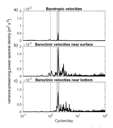
**Figure 2.4**: Variance-preserving power spectral density  $[m^2 s^{-2}]$  of total cross-shore (a) barotropic velocities, (b) baroclinic velocities near the surface (z = -4 m), and (c) baroclinic velocities near the bottom (z = -18 m). The dashed lines show the diurnal and M2 frequencies, with the frequency band used to isolate the M2 tide (Fig. 2.5E) in grey.
