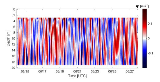
Figure 2.6: Low-pass filtered (< 1 cycle per hour) cross-shore velocities  $[m \ s^{-1}]$  measured at the ADCP during the full 14-day deployment. The black triangle shows the time of the M-AUE deployment. Positive velocities are onshore.
