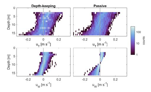
**Figure 3.3**: (Top) total and (bottom) wave-induced cross-shore velocities  $[m \ s^{-1}]$  for both (left) depth-keeping and (right) passive organisms in the simulated weakly nonlinear internal waves observed (n = 538 waves, 14 depths). The logarithmic colorbar shows the number of counts in each bin. Bins are 0.01 m s<sup>-1</sup> in size. Open circles show the M-AUE data, while the grey vertical line shows no velocities.
