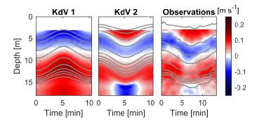
Figure 2.7: Observation and model comparisons. The background velocity profile in KdV 1 has the velocity measured at 3-m depth held constant to the surface, while in KdV 2 the background vertical shear measured at 3 m is extrapolated to 2.5-m depth, with velocity then held constant to the surface. Red colors are positive onshore and in the direction of the wave propagation. The grey lines show isopycnals every 0.15 kg m<sup>-3</sup>.
