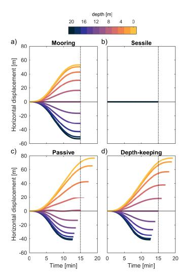
**Figure 4.3**: Horizontal displacement [m] from 0-20 m depth, (a) as predicted from the Eulerian velocities associated with the weakly nonlinear internal wave in Fig. 4.1, and for (b) sessile, (c) passive, and (d) depth-keeping organisms in the same flow field as in (a). The horizontal line shows no net horizontal transport, while the vertical dash-dot line shows the wave period. Colors show depth.
