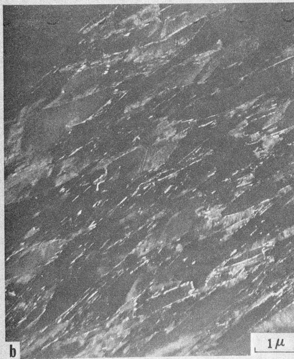
Fig. 17. Transmission electron micrographs of 4340, direct oil quenched from 1200°C, showing retained austenite films surrounding martensite laths: a) bright field image and b) dark field image of austenite reflexion showing reversal contrast of austenite films (after Lai et al. 6 ).
