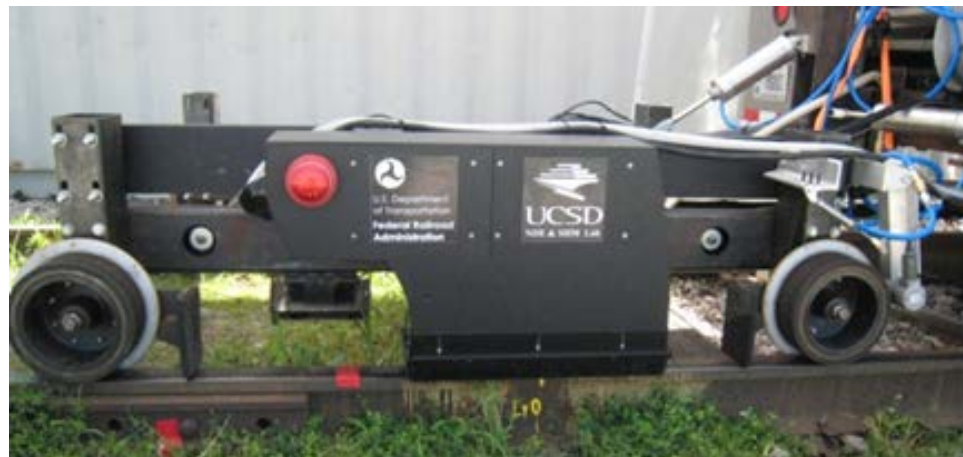
Figure 6-4: Rail Inspection Prototype Shoe and Cart
