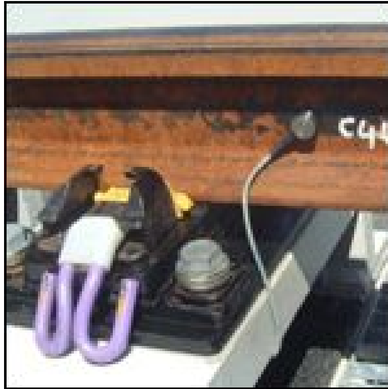
Figure 3-23: Stress Measurement by Inclusion Dilation Device
