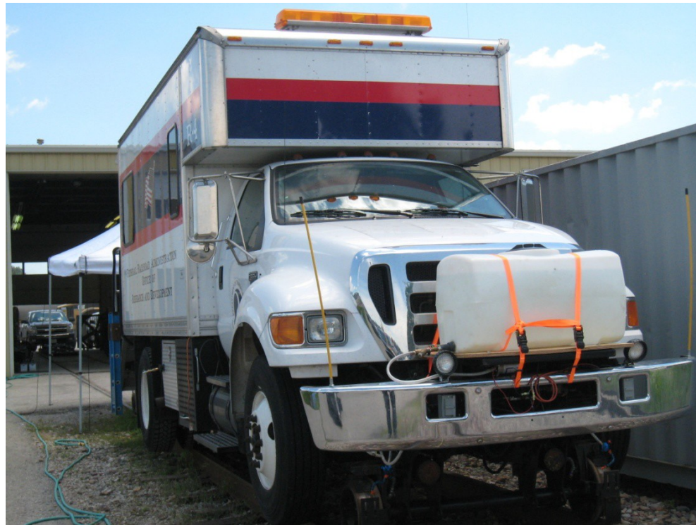
Figure 6-29: Water reservoir for the supply of the water spray system installed to reduce the noise created at the wheel-rail interface
