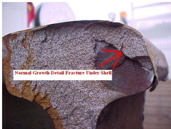
(a) Detail fracture (Tache Oval) under shelling (b) Detail Fracture with no Shelling
