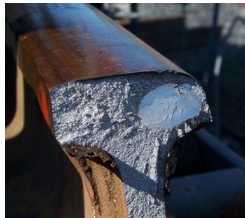
(a) Detail fracture (Tache Oval) under shelling (b) Detail Fracture with no Shelling
