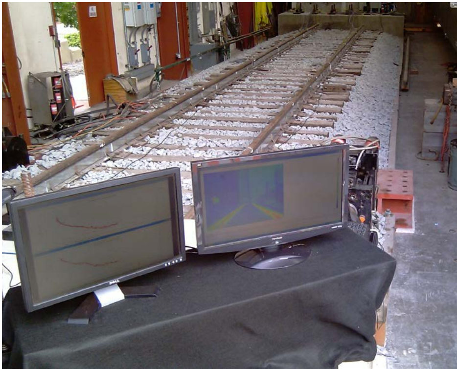
Figure 7-28: Completed Rail Neutral Temperature Test Platform
