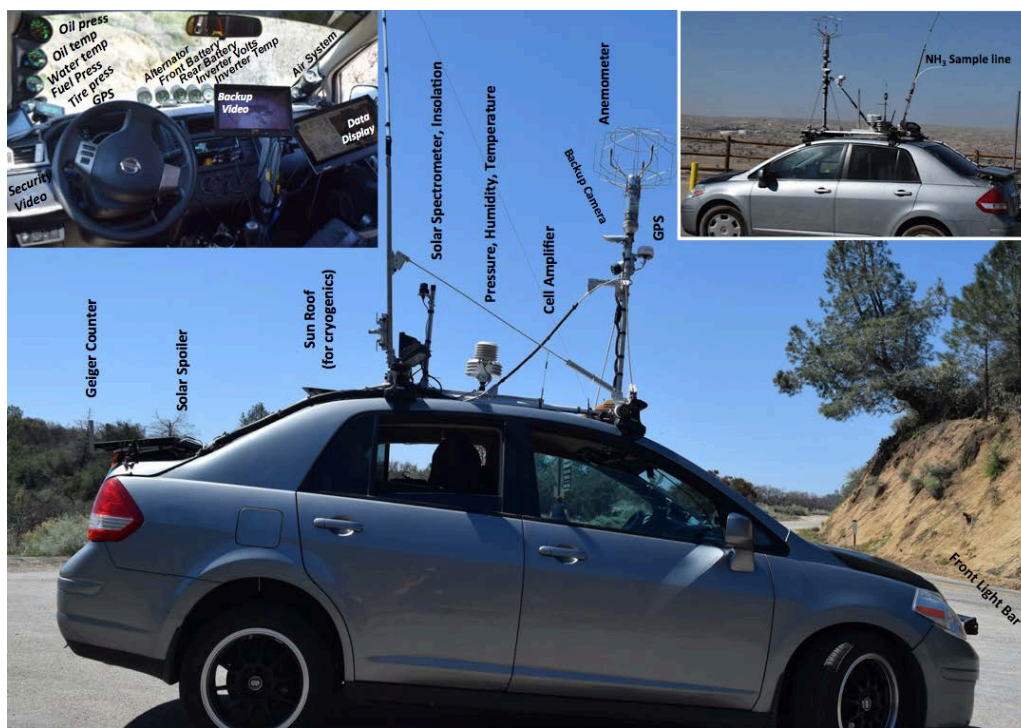
192 193 Fig. 1. Photos of AMOG (AutoMOBILE trace Gas) Surveyor. Upper left inset shows cockpit.
