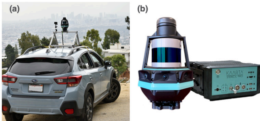
Figure 8. (a) Sensor Kit Mounted on the Car, (b) Perception Kit Showing GPS, LiDAR, and a Panoramic Camera
