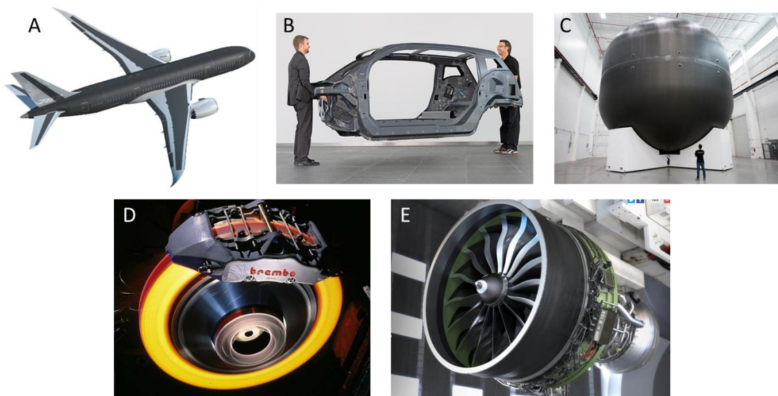
Figure 1.2. Examples of composite materials used in current and future aerospace and automotive structures. (A) Schematic of Boeing 787 Dreamliner highlighting use of CRFP laminates in the fuselage, wings, and tail. (B) BMW i3 passenger cell composed of CRFP. (C) CFRP liquid oxygen fuel tank for SpaceX's ITS rocket. (D) Formula One brake disc featuring carbon/carbon composite. (E) General Electric GE9X turbofan aircraft engine featuring CFRP fan blades and case as well as ceramic matrix composite nozzles and shrouds. Panel A adapted from Reference (4); panel B adapted from Reference (5); panel C adapted from Reference (6); panel D adapted from Reference (7); panel E adapted from Reference (8).
