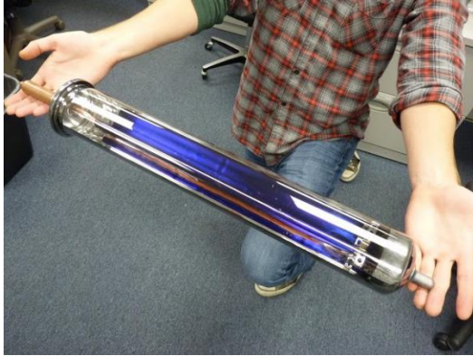
Fig.25 The ICPC half meter prototype, on the right, the icecream cone cross section of the absorber for the ease of fabrication.
