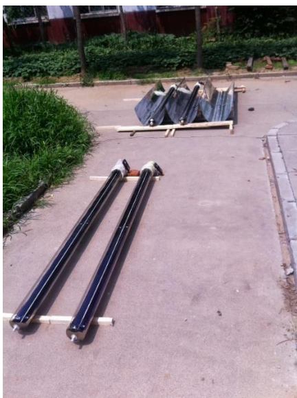
Fig.8 Test between flat absorber evacuated tubes and XCPC.
