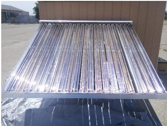
Fig.25. a) The ICPC 3.5m2 prototype, with full 1900mm length tube, front view.
