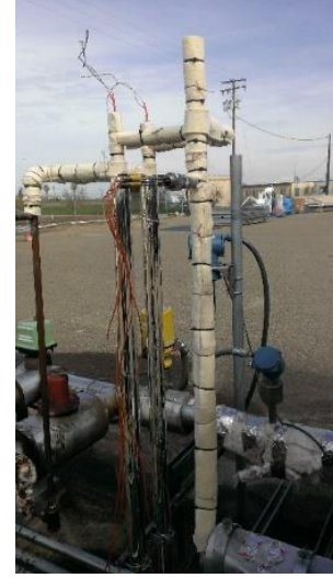
Fig 8. The calorimeter design (a.left) and its insulation process utilizing two vacuum tubes (b.right).
