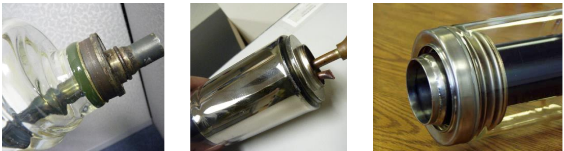
Figure 22 From left to right: housekeeper seal, thermal compression seal (the silver color inside of the tube is the barium getter), and the double end seal using bellows for the UVAC series tubes.
