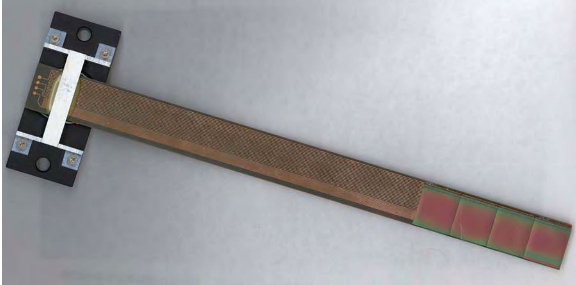
Figure 55: Mechanical Prototype with 4 MIMOSA-5 detectors glued to the Kapton cable assembly.
