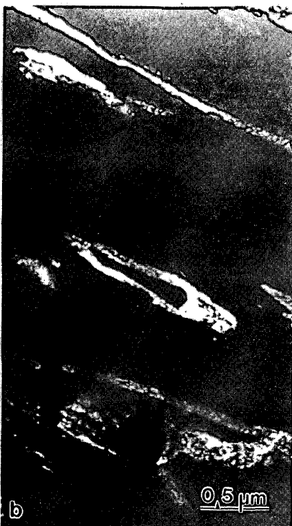
Fig. 10 Electron microscopy showing as cooled structure of QT 10 steel: (a) bright field, (b) dark field- interlath austenite, (c) darkfield- intralath M_3C .
