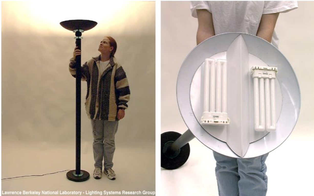
Figure 1: An example of a CFL Torchiere based on LBNL prototypes that is now available in the marketplace. The luminaires are similar in look to halogen torchieres, but they use two fluorescent lamps in a white reflector dish (as seen on right).
