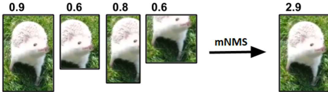
Figure 5.2: In modified non-maximum suppression (mNMS), the strongest bounding box is assigned with the cumulative sum of the scores of all overlapping neighbors.
