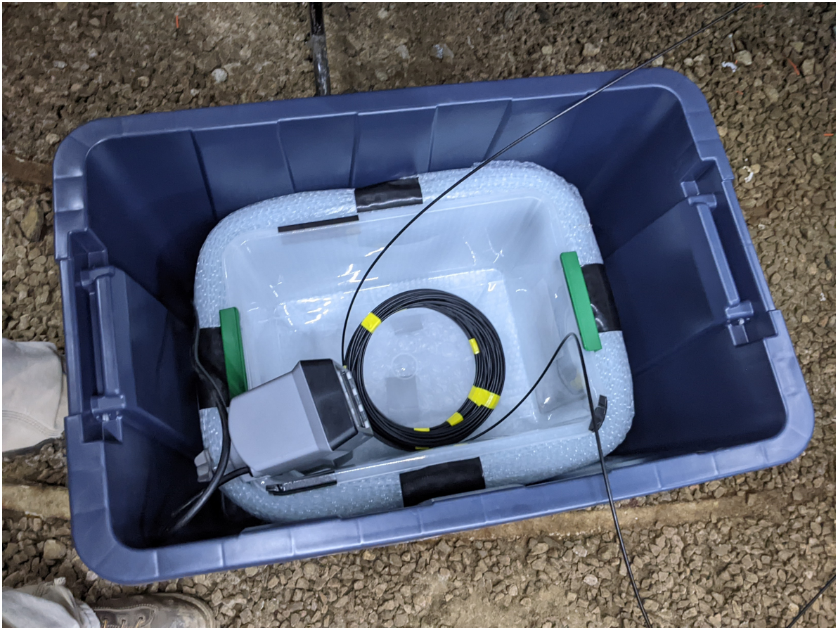
Figure 3: Interior of the hot water calibration bath showing the submersible heater (black) placed into the interior bath containing the fiber loop. This smaller bath was filled with water, capped, and then the entirety of the larger tub was filled with bubble wrap that acted as insulation.
