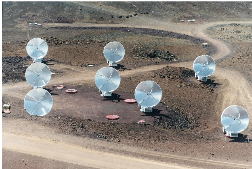
Figure 7.2: The Sub-Millimeter Array (SMA) on Mauna Kea, Hawaii. The interferometer consists of eight antennas and is able to operate at wavelengths as short as 0.3 mm.
