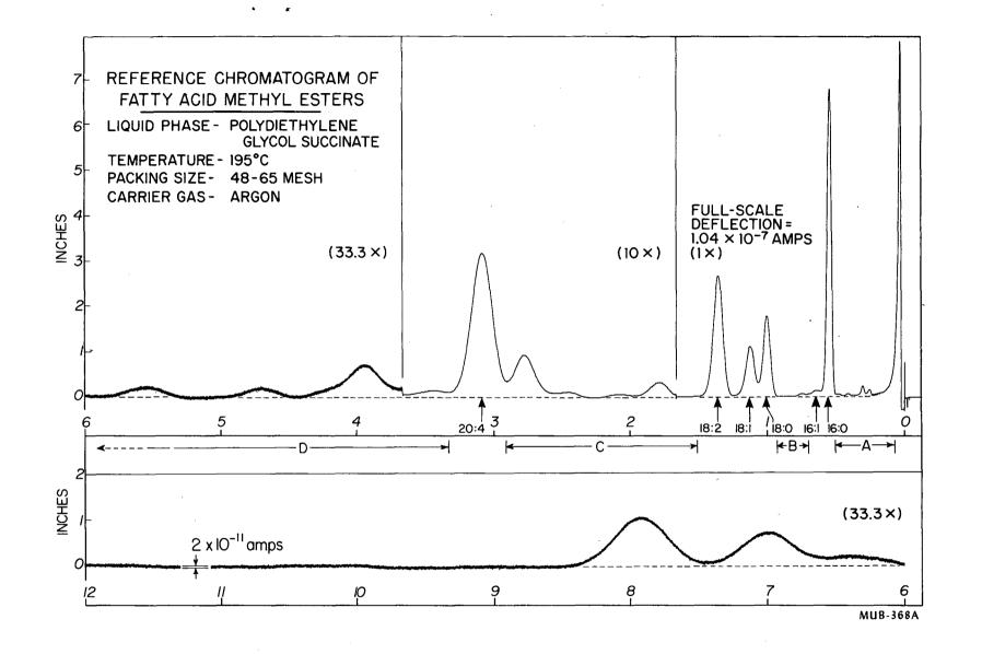
Fig. 1. Reference chromatogram of fatty acid methyl esters showing elution properties of known major components. Relatively minor components are grouped into four classes A, B, C, and D as indicated on the elution time scale. The elution time scale is marked off in units of methyl stearate elution times. .15-
