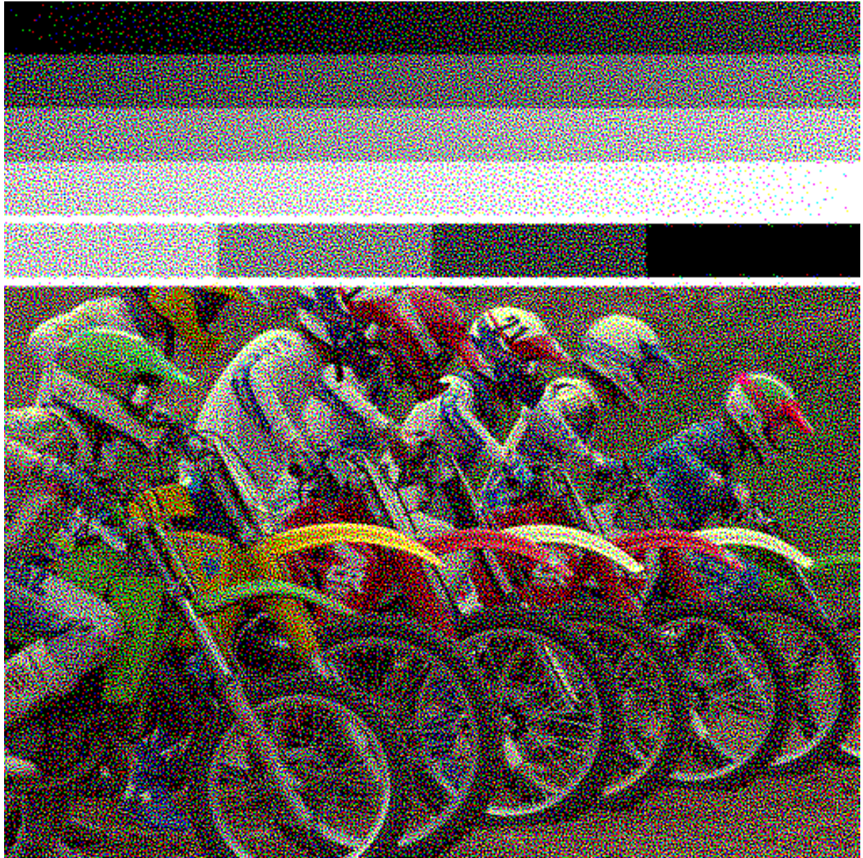
Figure 10. A 512 \times 512 halftone image generated using a inter-plane coefficient value of 0.2. With randomized intra-plane error filter weights. The pinwheel image block size: 10 \times 10 . Both grain and block-shape periodic patterns are mitigated.
