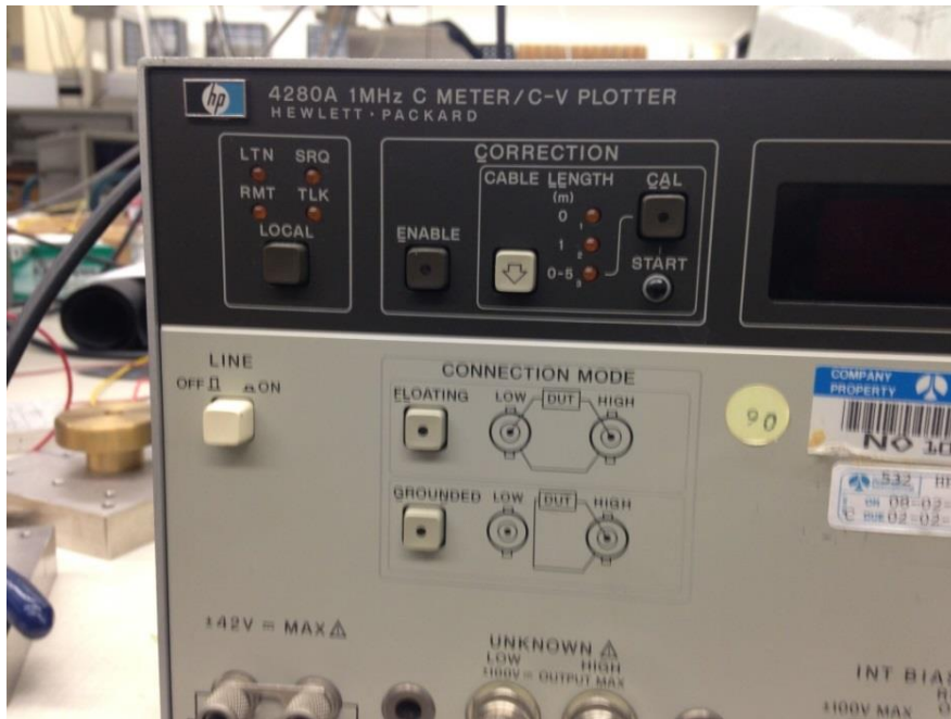
Fig. 4. 1. HP 4280A 1MHz C Meter / C-V plotter used for capacitance measurement.
