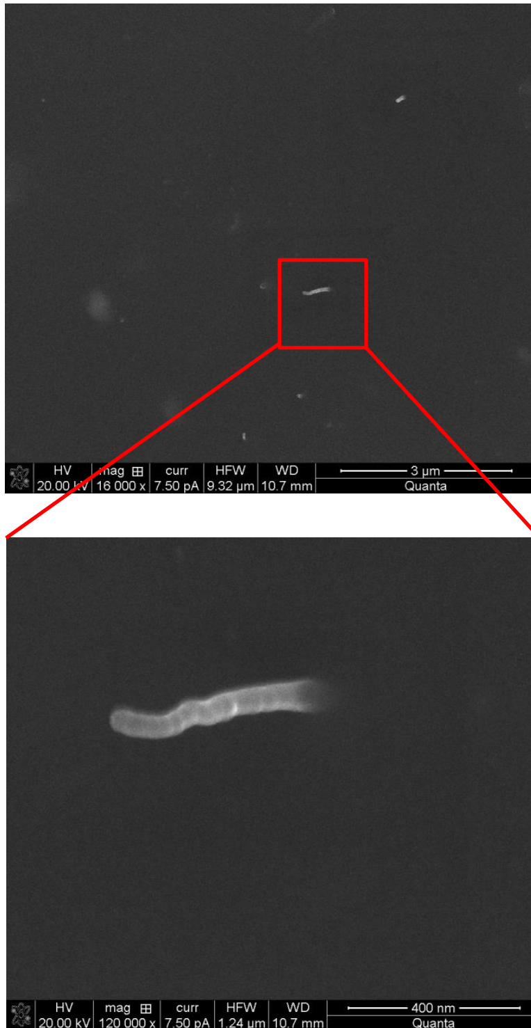
Fig. 2. 9. SEM images of nanocomposites with 0.3 wt. % MWNTs processed with acetone with 4.0-hr ultra-sonication treatment.
