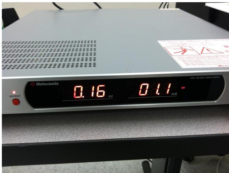
Fig. 3. 19. Power supplier (Matsusada AU-10P30-LC) used in the displacement measurement by laser Doppler vibrometer.
