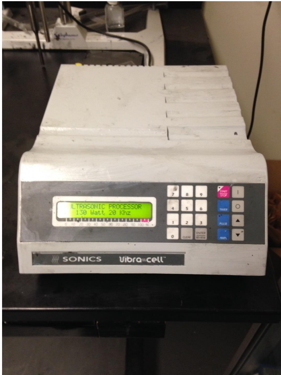
Fig. 2. 2. VCX 130 ultrasonic distributor for ultra-sonication processing.
