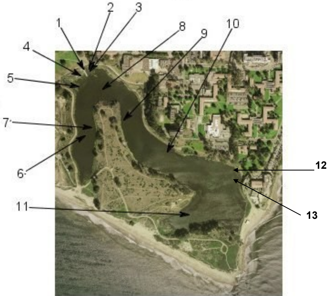
Figure 1. Dissolved oxygen sampling sites. Sites were sampled in the morning (6-7am) and in the afternoon (3-5pm) on a biweekly or slightly less regular schedule at the surface, 1 meter from the surface and the bottom (~ 2.5 m) using a YSI 85.
