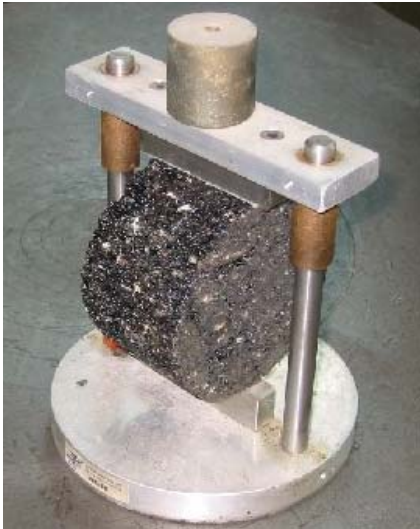
Figure 5-13 Equipment used for the TSR test (a – Southwark Tate-Emery hydraulic testing machine, b – Gilson MS-35 Lottman breaking head)
