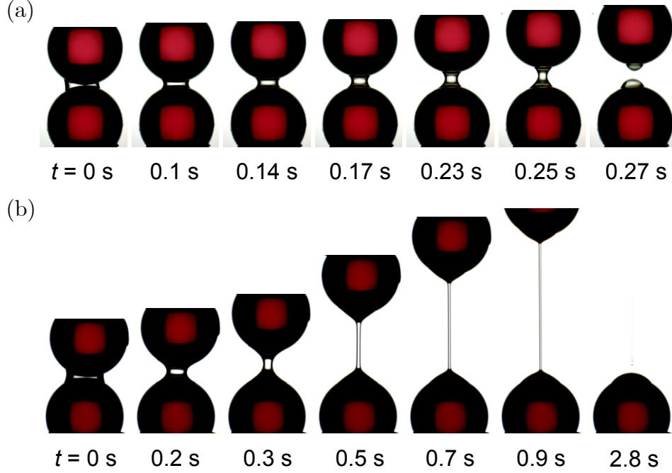
FIGURE 1.7: Thinning of a liquid bridge of (a) Water, and (b) PEO of M_w = 4000 kg/mol with 1% by mass concentration prepared in water. The liquid bridge is positioned between two beads of radius R = 2 mm and separated with a velocity, v = 10 mm/s.
