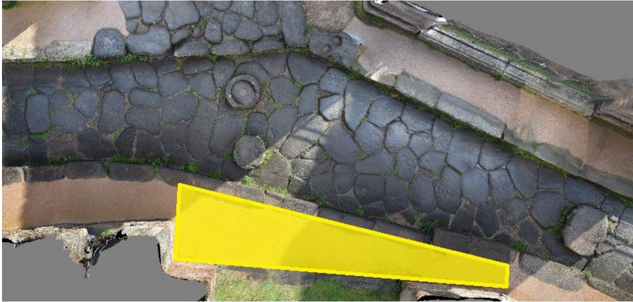
Figure 37 - Photogrammetric model showing the sidewalk widening in front of Casa dell'Orto Ferito to accommodate crossing from the south.
