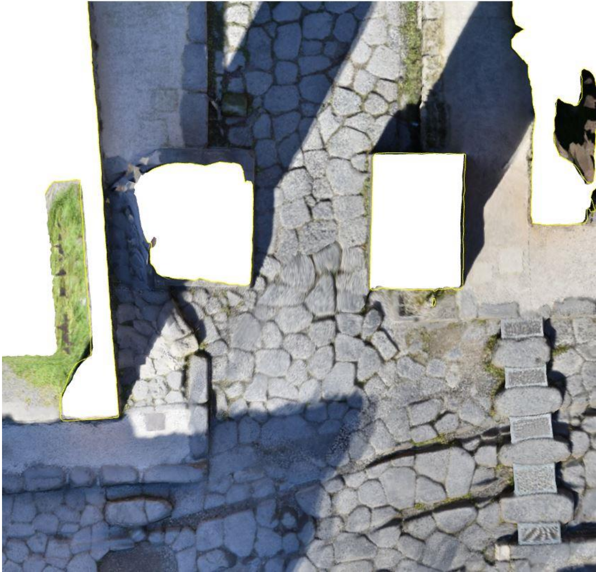
Figure 47 - Image-based model of Intersection G with a horizontal section through the Arch of Caligula, highlighting the severe bottleneck to pedestrian and vehicular traffic caused by the piers of the arch..
