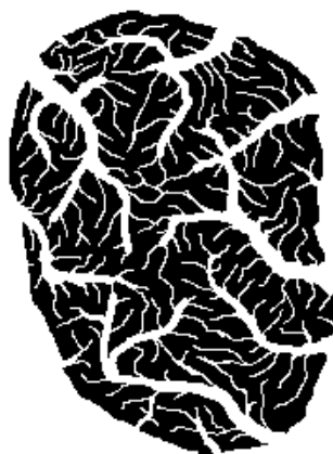
Figure 6.5. Illustration of a section through an activated carbon particle, showing a conceptual representation of the pore structure. Image taken from http://www.roplex.co.uk/carbon_adsorption_vru.htm
