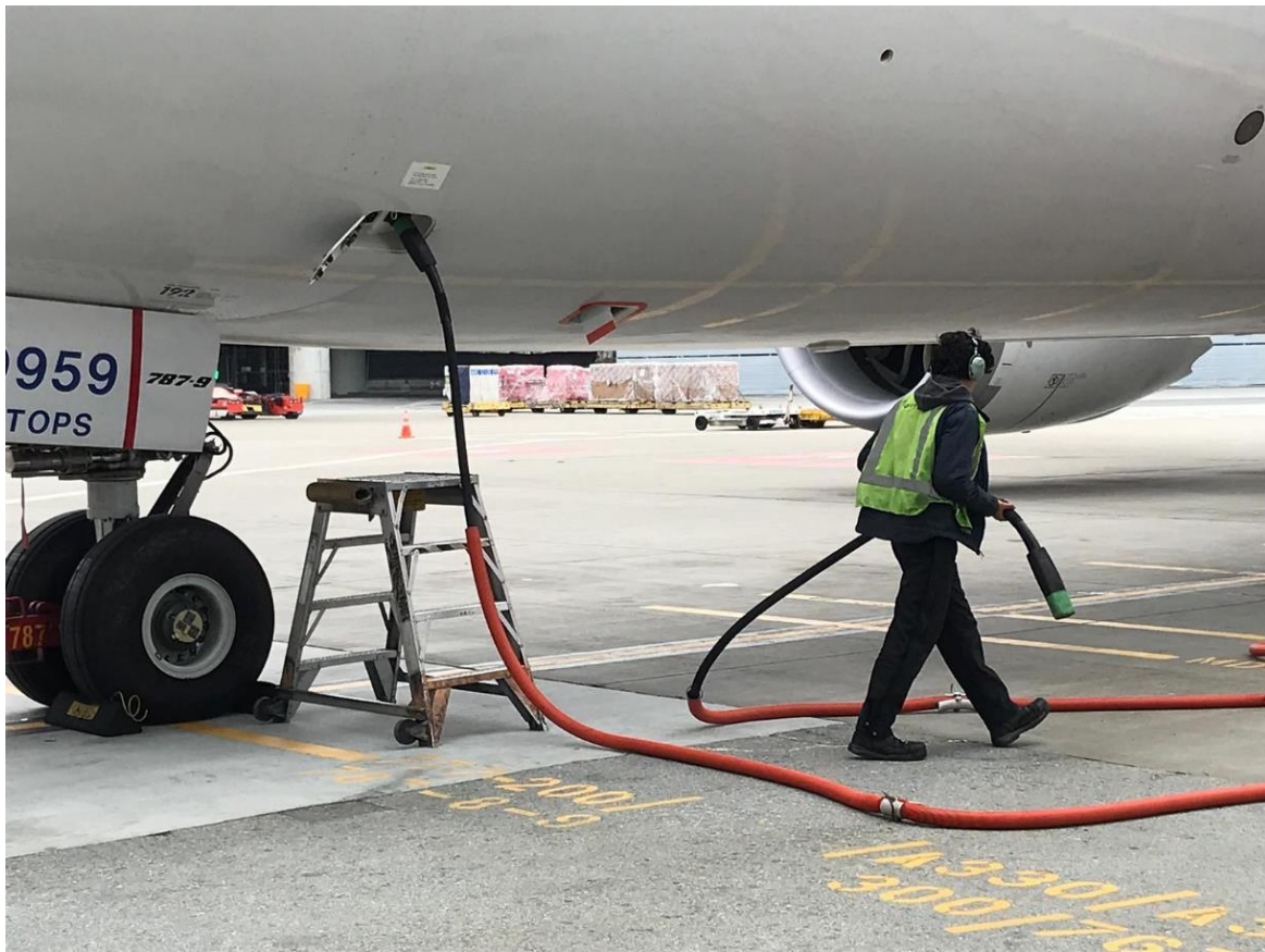
Figure 36: Ground crew worker disconnects a GP cable from a 787-900 which requires 2 GP cables for higher current supply (Achatz Antonelli, 2019)
