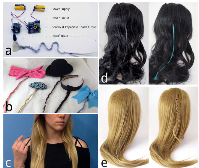
Figure 1. A) HäiriÖ prototype prior to miniaturization, B) exemplar HäiriÖ hair accessory form factors, C) HäiriÖ uses Swept Frequency Capacitive Sensing to detect natural hair interactions, D) HäiriÖ color changing properties using thermochromic pigments, and E) shape changing properties using Nitinol wire.
