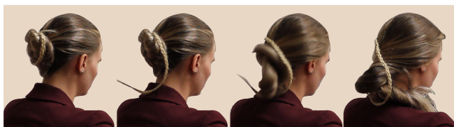
Figure 7. Physical implementation of application. HäirIÖ braid is twisted around a bun. Upon actuation, the braid begins to straighten out, unwrapping from the bun and falling on the user's shoulder. A second wire unravels similarly, and the entire bun falls down. This technique also employs haptics, as the hair movement elicits a tactile sensation.
