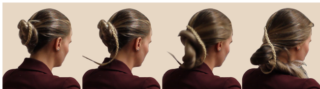
Figure 7. Physical implementation of application. HäirIÖ braid is twisted around a bun. Upon actuation, the braid begins to straighten out, unwrapping from the bun and falling on the user's shoulder. A second wire unravels similarly, and the entire bun falls down. This technique also employs haptics, as the hair movement elicits a tactile sensation.
