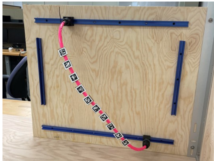
Figure 34: Apriltags used to obtain ground truth position of wire
