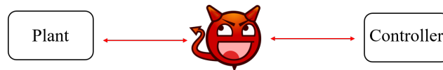
Figure 1.7: The man in the middle attack: the attacker acts as a malicious controller for the plant and a fictitious plant for the controller
