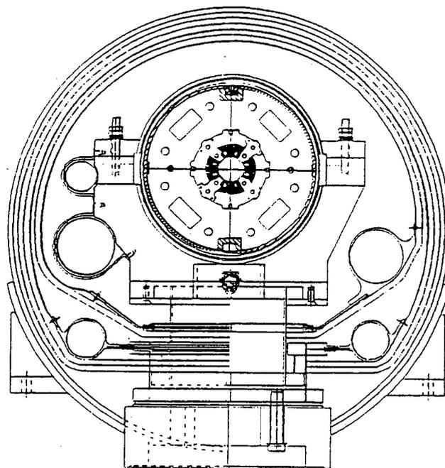
Figure 6. Cross section of complete magnet showing the cold mass mounted in the cryostat.
