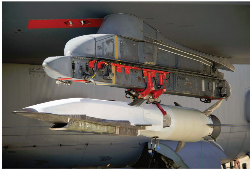
Figure 1.1: The X51-A hypersonic test vehicle mounted to the wing of a B-52 bomber. The forward section is the scramjet-powered vehicle, while the region behind the first set of fins is a booster rocket to accelerate the vehicle to Mach 4. The scramjet engine comprises most of the lower section of the vehicle: approximately the full region with a metallic finish. (Wright-Patterson Air Force Base, 2012)
