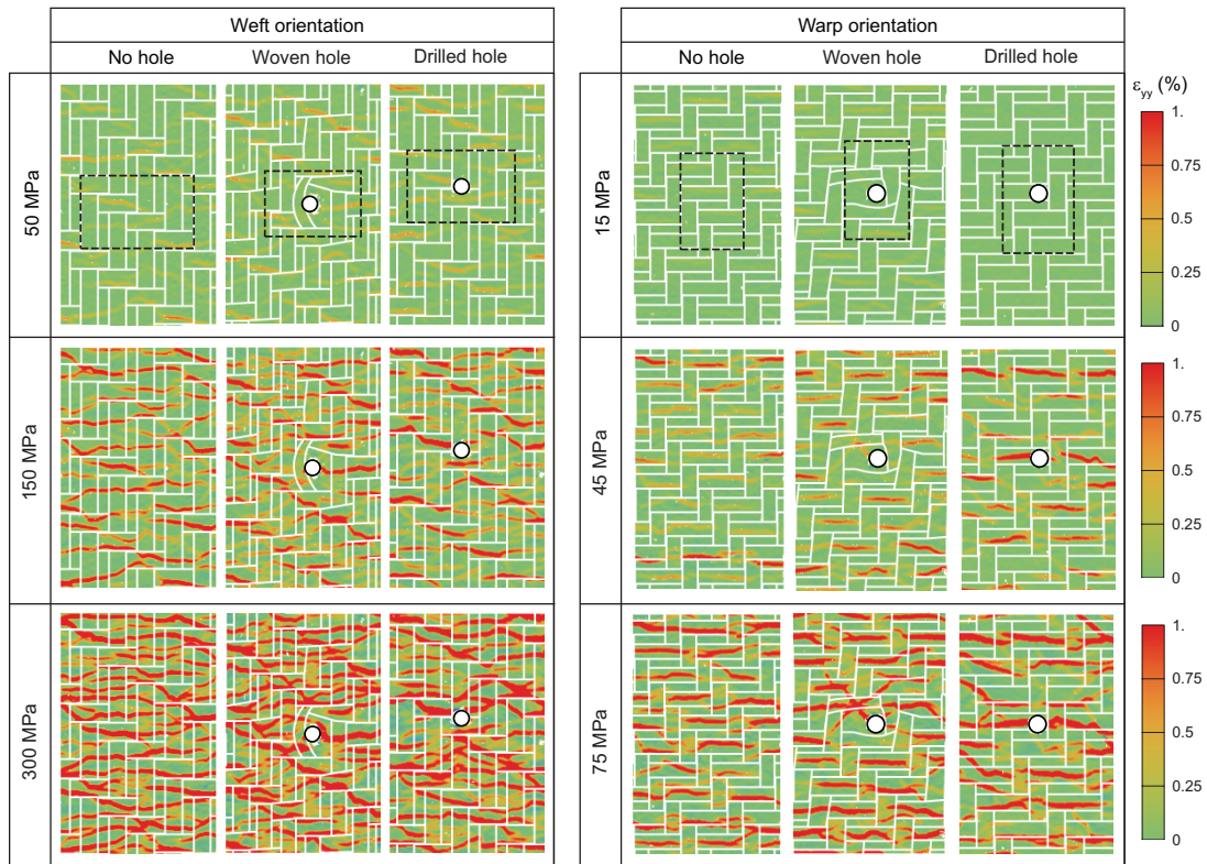
Figure 5.7: Full-field axial strains of tensile specimens in weft and warp directions at the stress indicated for specimens containing holes. Underlying tow boundaries are overlaid in white. Dashed rectangles represent the unit cell. Full-field axial strains of the pristine composite have also been plotted for reference.
