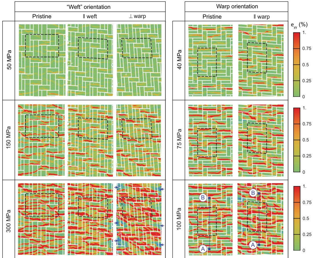
Figure 5.11: Full-field axial strains of tensile specimens from the sheared composite panel in the (nominally) weft and warp directions. Underlying tow boundaries are overlaid in white. Dashed rectangles/parallelograms represent unit cells. Equivalent contour plots for the pristine specimens have been included for reference. Points A and B denote the end points of the line scan plotted in Fig. 5.14. Arrows in the bottom image of the center column denote near-edge regions where the axial strains are essentially zero. (Note the slight differences in image magnification for the various test specimens.)
