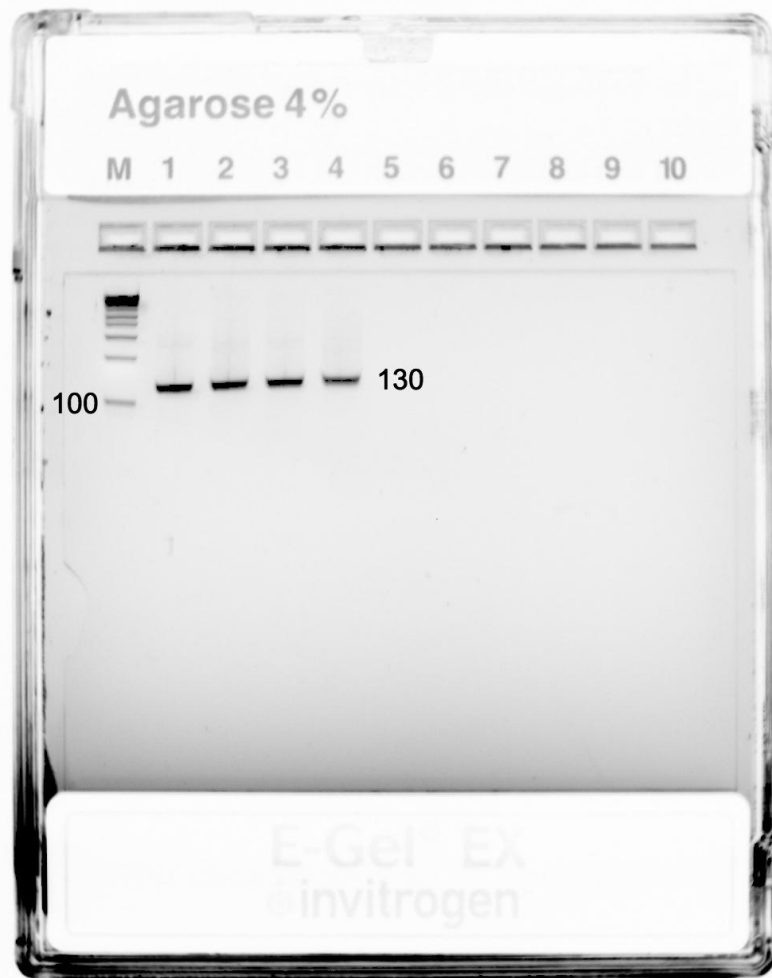
Figure 4. 4% agarose E-gel used to check the length of the adapter after PCR. Bottom of the ladder corresponds 100bp, adapter length is ~130bp.
