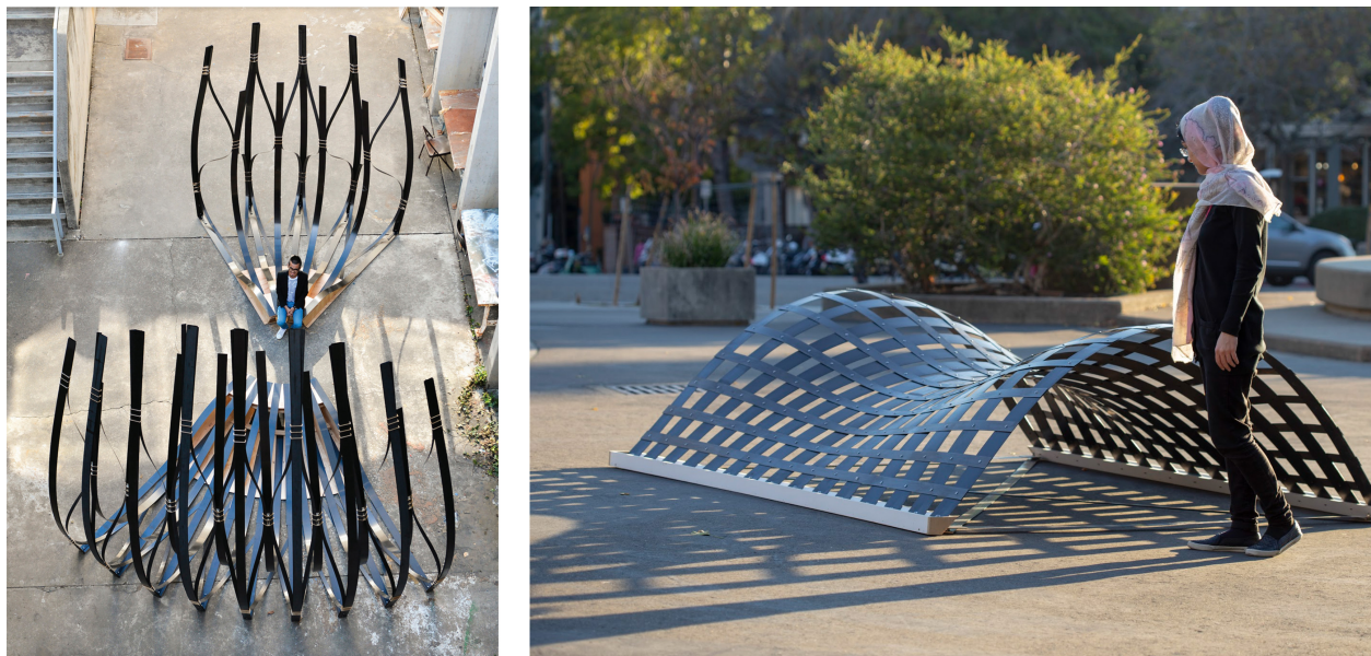
Figure 3.1: Left: Feasibility study on gaining stability from flexible material Right: CFRP bending-active formwork for the construction of concrete shells.
