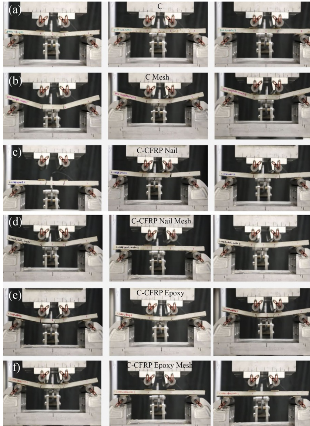
Figure 4.7: Beams after performing the four-point bending test (each row, from left to right): (a) C 1-3 (b) C Mesh 1-3 (c) C-CFRP Nail 1-3 (d) C-CFRP Mesh Nail 1-3 (e) C-CFRP Epoxy 1-3 (f) C-CFRP Epoxy Mesh 1-3.
