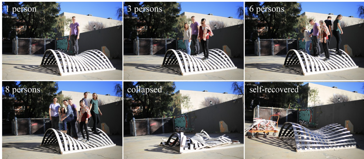
Figure 3.13: Ultimate loading test reveals the shell's resilient behavior.
