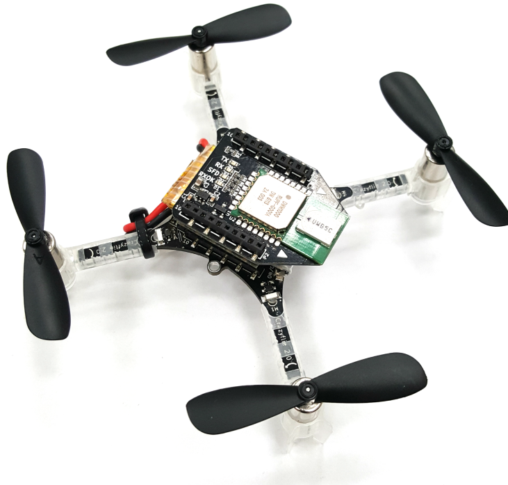
Figure 2.3: The quadcopter used in our experiments as the mobile agent. The UWB ranging sensor (seen in this picture) works at the rate of approximately 60 Hz.
