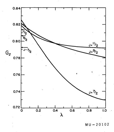
Fig. 4. Calculated  $g_I$  factors of the levels J=11/2, 9/2 and 7/2 of Pa as a function of the strength of the electrostatic interaction.
