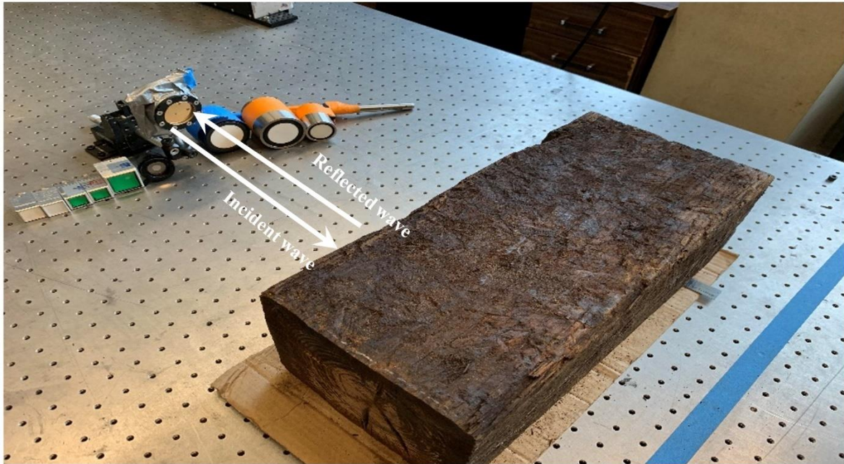
Figure 5.7 Array of piezoelectric and capacitive transducers tested at UCSD
