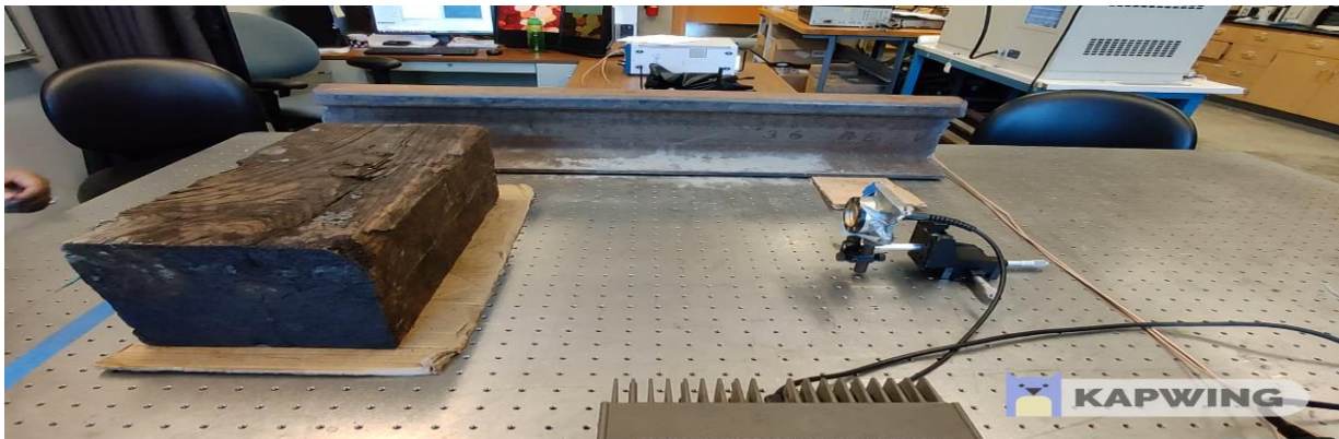
Figure 5.9 Tie-sonar experimental setup using one transducer in pulse-echo mode on wood tie
