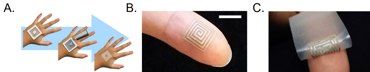
Figure 5.3 Visualization of the conductive Ag ink tattoos. A) Process flow for patterning the Ag ink onto the skin using a disposable adhesive stencil mask. B) Example of an Ag ink tattoo patterned over the fingerprint region of the index finger. Scale bar is 1 cm. C) Removal of the Ag ink tattoo via adhesive tape shows impressions of the papillary ridges.
