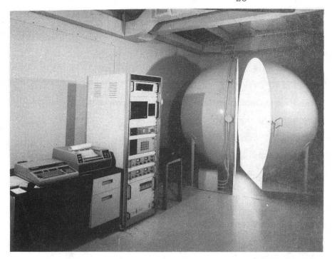
Eight-foot integrating sphere with data acquisition system.
