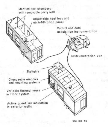
Schematic view of Mobile Window Thermal Test (MoWiTT) facility.
